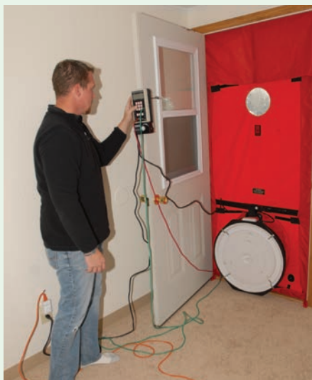
A tribal member practices setting up and operating a blower door during an energy audit training at the tribal sports arena, Chi-Mukwa. Photo from Kathie Brosemer, Sault Ste. Marie Tribe of Chippewa Indians, NREL 32756
